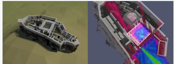
Figure 3a. 3D transparent reconstructed walls on top of the dense 3D mesh captured using photogrammetry.
